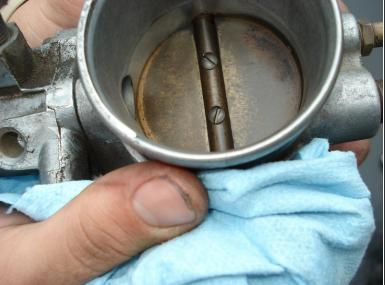
Cover the electrical contacts with a shop towel to prevent throttle body cleaner from inadvertently spilling over.
