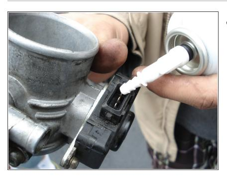
Apply a small amount of dielectric grease to the metal contacts to prevent corrosion.
