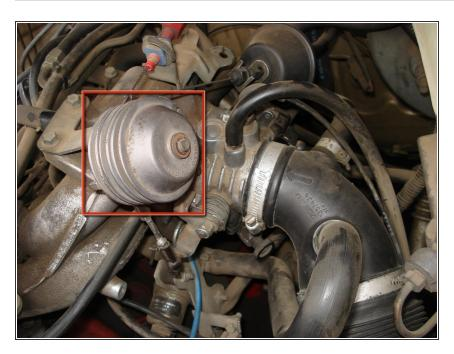
Locate throttle linkage cable assembly.
