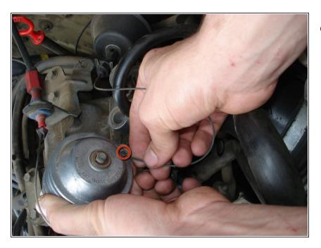
Slide both slackened cables off assembly's guides.
