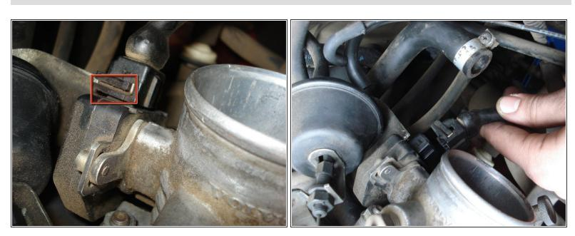
Press down on the locking mechanism before gently removing the wiring clip.
