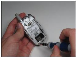
• At the corners of the phone, remove all four 6.0 mm Torx screws, using your screwdriver.
