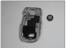
• Separate the speaker from the casing by pushing with a pin from the back (external) side, through the openings in the casing.
