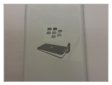
Remove the battery cover by grabbing the notch under the bottom speakers and lifting.
