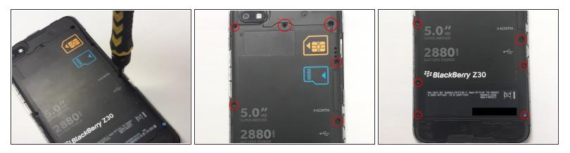
• Locate and unscrew all 10 T5 screws around the back cover
