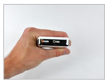
Before opening your iPod, ensure that the hold switch is in the locked position. The orange bar should be visible, indicating hold is active.
