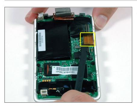
Use a spudger to carefully disconnect the orange touch wheel cable from the logic board.
