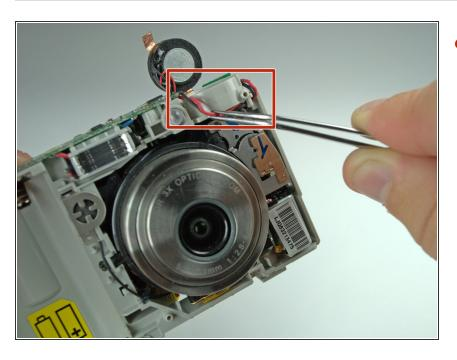
Pull the wiring at the top right of the camera away from the lens with tweezers.
