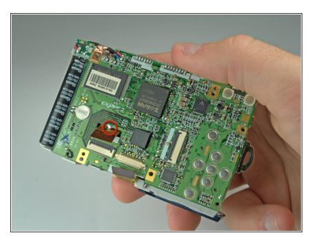
Desolder the connection of the motherboard to the lens ribbon using a soldering iron and desoldering wick.
