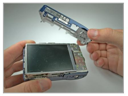
Pry the back cover from the left side of the camera. Remove the cover gently.
