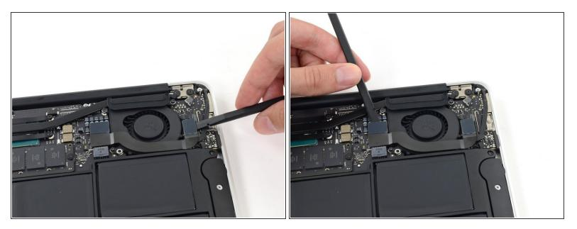
Use the flat end of a spudger to pry the left and right I/O board cable connectors up off their respective sockets on the I/O board.
