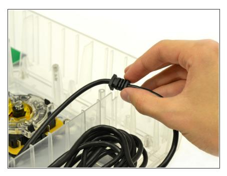
Slide USB cable up from the plastic barrier casing.
