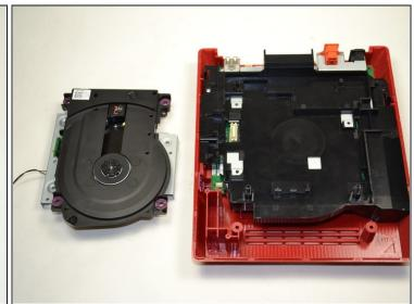
• Lift the disc drive out of the console and set it aside.
