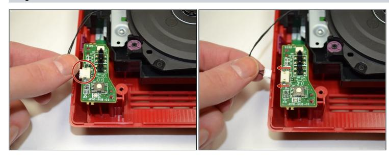
• Using your fingers, gently pull the pin connector to disconnect the power board from the disc drive.
