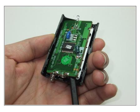
Gently use the spudger to pry the circuit board loose.
