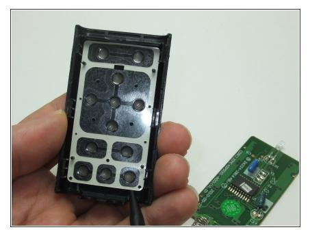
Using either end of the spudger, gently lift and remove the clear keypad backing.
