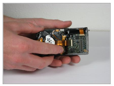
• Push the lens assembly slightly toward the circuit board, and pull the left side out of the casing first. You will have to wiggle this out gently.
