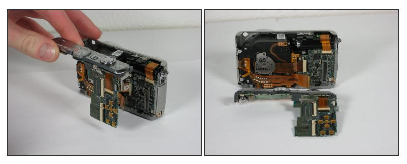
Slide the entire top part of the camera that is attached to the logic board, horizontally away from the camera.
