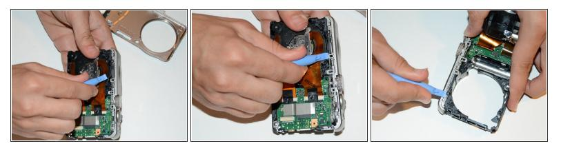
Release the top cover by lifting several tabs with the plastic opening tool. Go gently to avoid breaking them.
