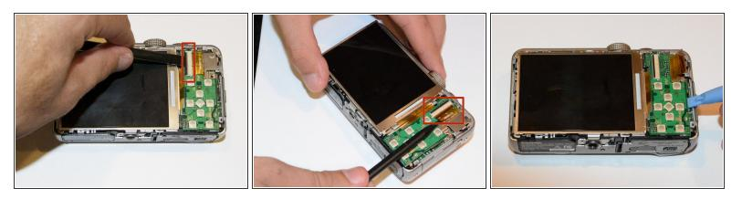
• Use a spudger to lift the LCD ribbon cable locking bar by angling it up, then withdraw the ribbon.
