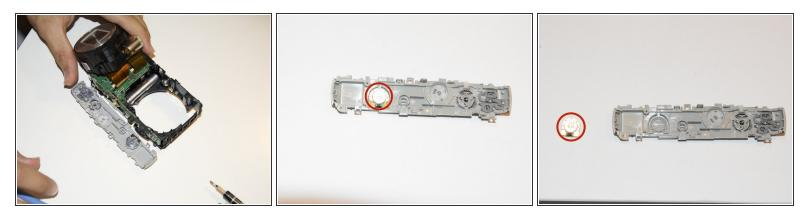
• With the top cover removed the speaker can be very easily removed or replaced.
