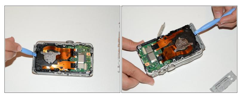
• Remove the side covers using the plastic opening tool.
