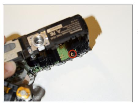
To remove the top cover, you need to remove a 3.7 mm screw as shown.
