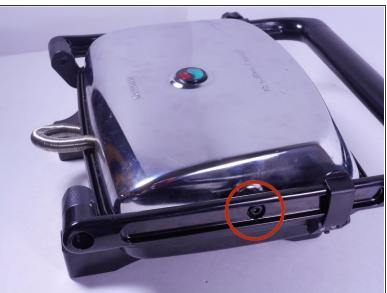
• Using the 4.0mm Allen Wrench, unscrew the two 26mm bolts connecting the handle to the upper heating element housing on both sides.
