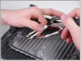
Nery gently, slide the white wiring covers down to expose the wiring connectors
