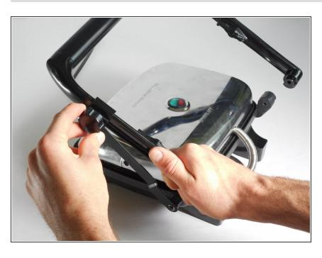
Unscrew the locking knob all the way to remove it.
