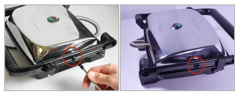
Using the 4.0mm Allen Wrench, unscrew the two 26mm bolts connecting the handle to the upper heating element housing on both sides.
