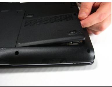
Remove the two screws from the hard drive shield and lift it off starting at the right side. The screws will remain in the shield.
