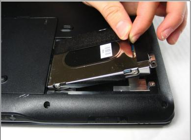
Pull the plastic tab attached to the hard drive. The hard drive lifts right out. Pull gently so you don't damage the contacts.
