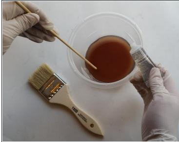
It's time to mix the resin and hardener together. Read the specific instructions on the back of the container to get the accurate ratio of resin to hardener.
