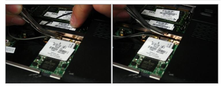
• Use a pair of <u>tweezers</u> to disconnect both antennas from their sockets on the wireless card.
