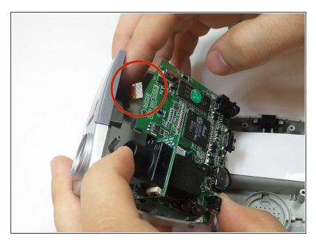
• Take out the motherboard while disconnecting the flip screen's cable from underneath.
