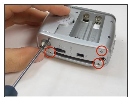
• Remove the four screws from the back side.
