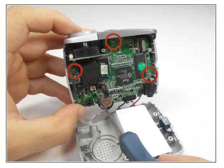
• Remove the four screws from the motherboard.
