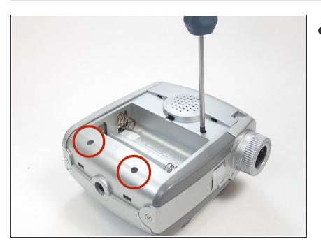
Unscrew the three 4mm screws from the battery side of the device. Use a Phillips screw driver.
