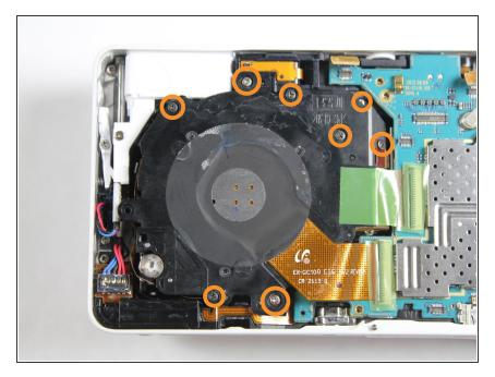
Unscrew the lens' screws. There are 1 black 4/32" screw, 3 3/16" black screws, and 2 white 5/32" screws.
