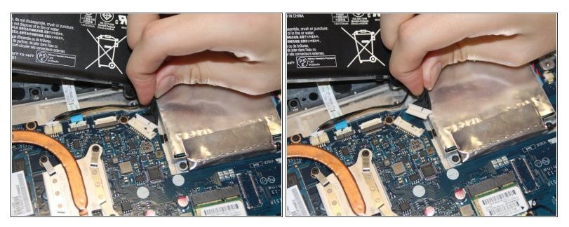
• Remove the battery cable from the motherboard by gently pulling out on the black part of the cable closest to the white tab.
