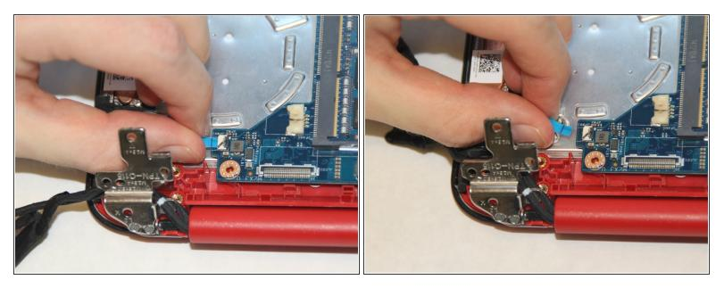
• Pull the cable horizontally away from the motherboard to disconnect the power button board cable.
