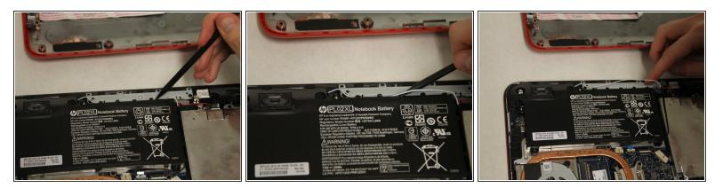
• Use the spudger to pry up the blue/white speaker wires that are routed beside the battery.
