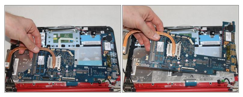
• Lift up to remove the motherboard.
