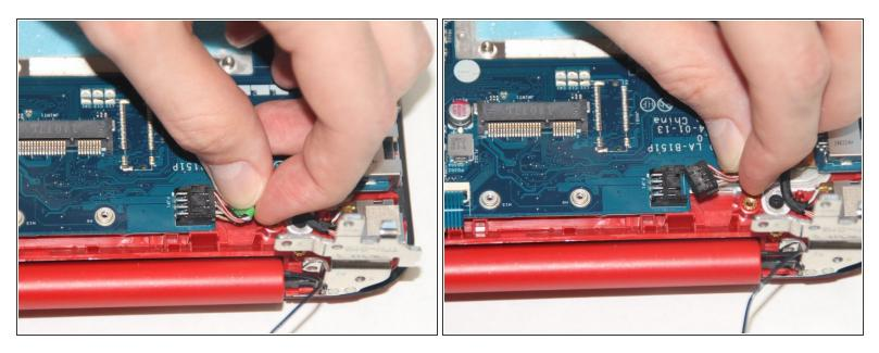
• Pull the cable horizontally away from the motherboard to disconnect the power connector cable.
