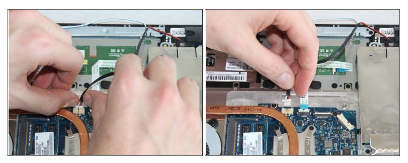
• Pull the cable horizontally away from the motherboard to disconnect the speaker cable.
