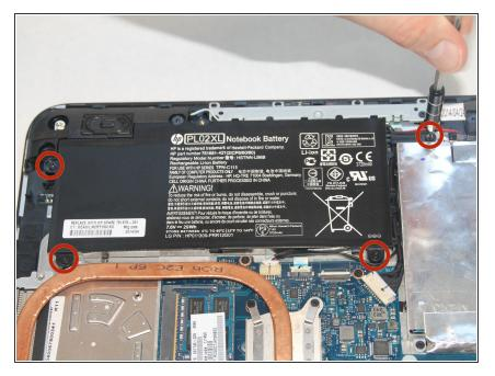
Remove the four 6mm screws from the battery with the PH0 screwdriver.
