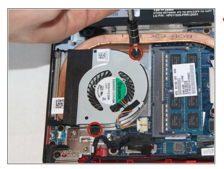
Remove the two 3mm screws with the PH0 screwdriver.
