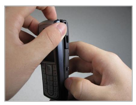
Slide your thumbnail down the case seam to separate the rest of the case.
