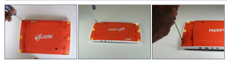
• You can remove the rear casing by unscrewing all six phillips #00(3.5mm x 4.5mm)screws from the left and right side of the device.
