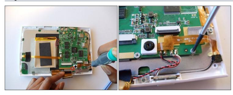
• Remove the two phillips #00 (4.5mm x 3mm)screws located on the motherboard.
