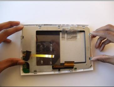
• Slowly remove the metal frame and screen from the white casing by gently pulling up on the ends of the metal frame.
