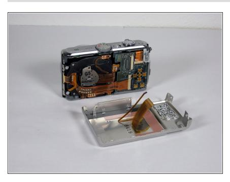
Remove the back casing from the camera.
