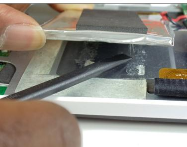
Use your spudger to separate the battery from the adhesive glue strips and plastic film.
