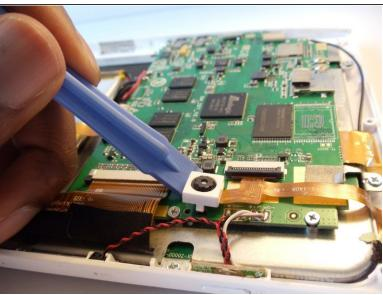
Slip the plastic opening tool under the white, square enclosure of the camera and lift upward to unhook the camera unit from the motherboard.
