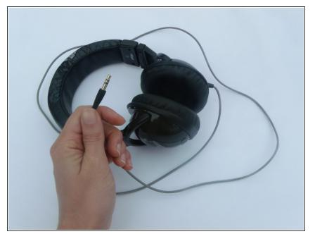
Gently gripping the auxiliary cable of your headset, run your fingers down it's length, feeling for bumps or tears in the plastic sheathing. If there are multiple damaged areas, choose the one closest to the device.
