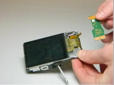
• Flip over the control board then use tweezers to pull out the ribbon connecting the circuit board to the motherboard.
