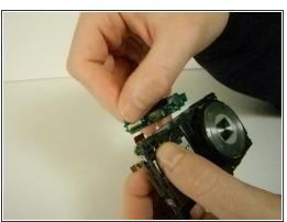
Once the case is off, hold down the ribbon near the LCD screen that connects the flash to the camera. While doing this, carefully lift the control board that contains the flash until the ribbon is no longer connected.
