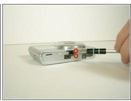
• Open the battery/memory card door and remove the 6 screws (.35cm) with a Philips 000 screwdriver. There will be two screws on the left and right sides, and two on the bottom.
