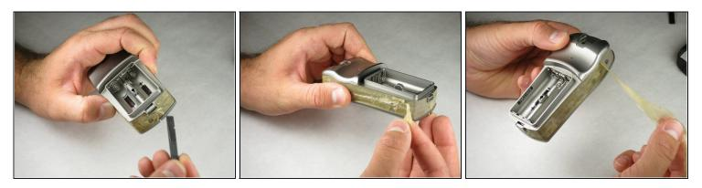
• With the pick side of a spudger (or <u>tweezers</u>), peel the sticky tape from the device.
