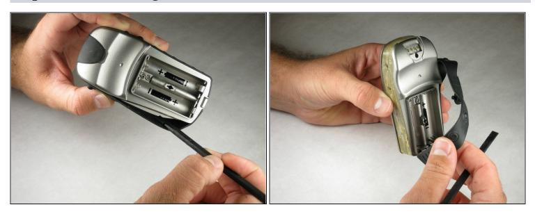
• With the wedge side of a spudger (or a small, flat head screwdriver), remove the black rubber case support from the device body.
