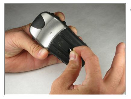
• Lift the metal tab up, and rotate it counterclockwise. This will unlock the back case cover.
