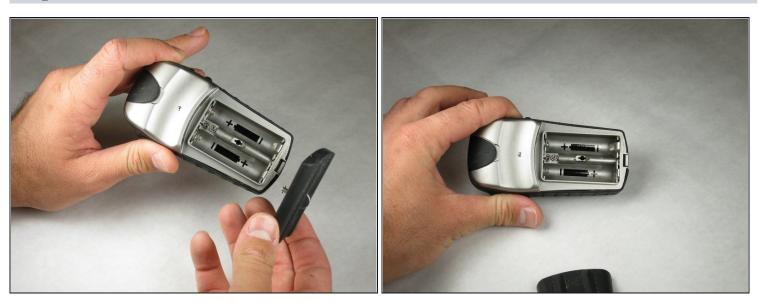
• Lift the battery plate off to either insert or remove 2 AA batteries.
