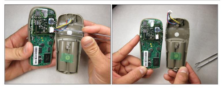
• With tweezers (or your fingernails), carefully disconnect the wires between the PC input and the motherboard.
