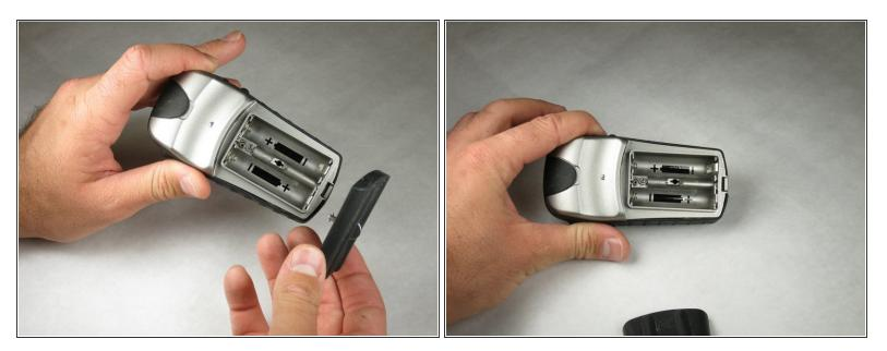
• Lift the battery plate off to either insert or remove 2 AA batteries.
