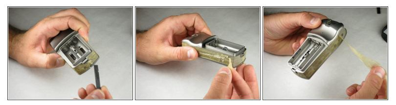
• With the pick side of a spudger (or tweezers), peel the sticky tape from the device.
