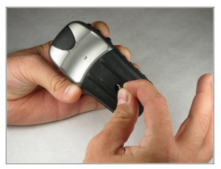
• Lift the metal tab up, and rotate it counterclockwise. This will unlock the back case cover.
