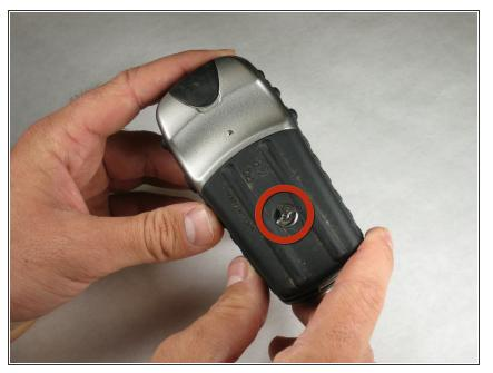
• Flip the device to the backside, and locate the metal tab at the center of the back cover.
