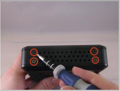
Unscrew and remove the eight 4mm Phillips #0 screws (four on top, four on bottom) from the top and bottom of the device.
