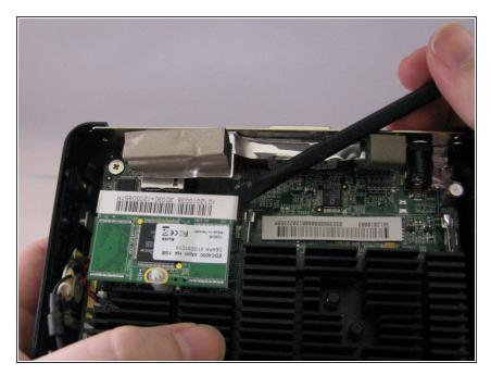
Using the spudger, gently push on the underside of the memory board to loosen it. Gently grasp each side and pull up to release the memory board.
