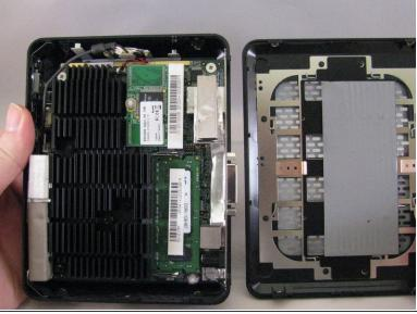
Once the clips have been released, gently disengage the cover from the rest of case by pulling in opposite directions.
