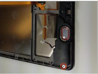
Use Phillips #0 screwdriver to remove two screws from either end of the speaker.
