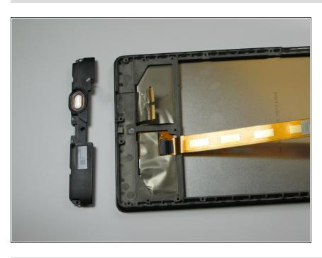
Carefully lift bottom speaker from the device.
