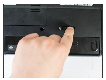
• Push the switch as far to the right as possible to unlock the battery.
