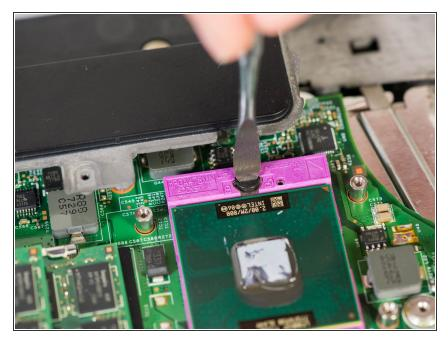
Use a Metal Spudger to turn the black plastic screw to the unlock position from the secure position of the CPU on the motherboard.
