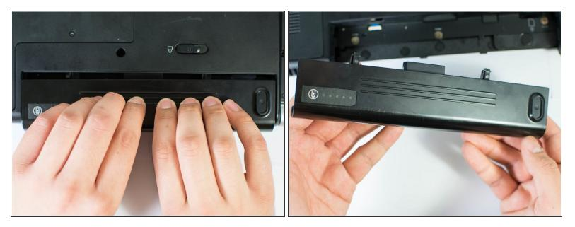
• Remove the battery using two hands and pull it away from the computer.
