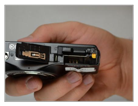
Swing the door open to expose the battery compartment.
