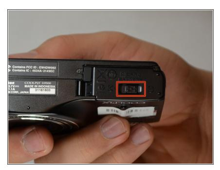
With the bottom of the camera facing you, find the battery latch and slide it to the left.
