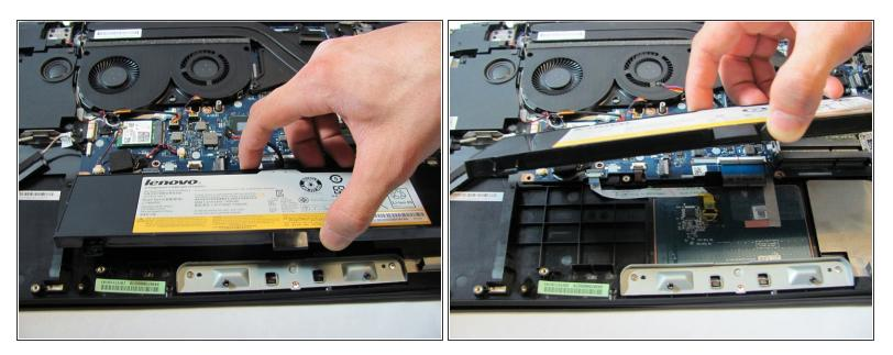
• Lift the battery out of the computer.
