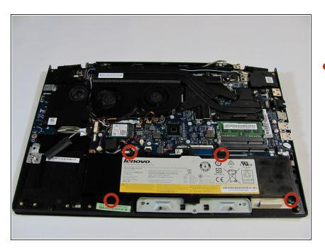
Remove all four 6 mm screws from the battery using the Phillips #1 screwdriver.
