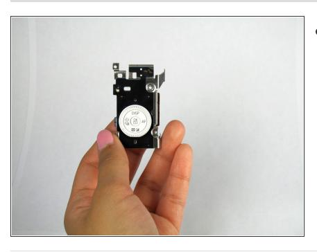
Remove the button assembly from the back panel
