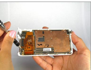
Remove all five 3mm Philips #000 screws from the inside of the back panel using the Philips #000 Screwdriver.
