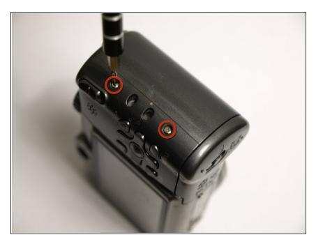
Remove the two screws located on the other side of the camera using a Phillips #00 screwdriver.
