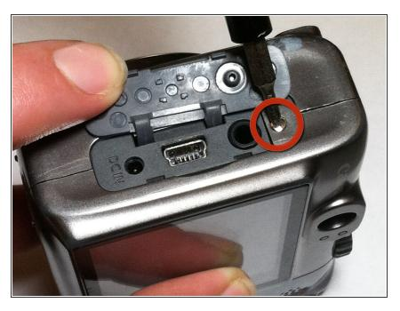
Remove the screw located under the rubber flap on the left side of the camera using a Phillips #00 screwdriver.
