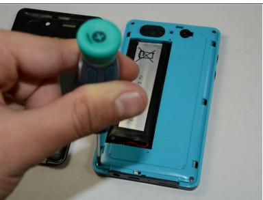
To remove the battery, make sure the four 5mm Philips screws on each side of your device is open using the Philips#1 Screwdriver.
