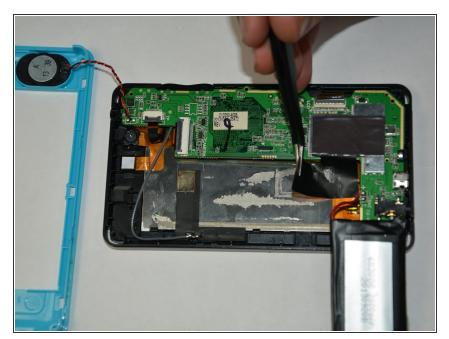
Use tweezers to remove the black tape that is attached to the motherboard.
