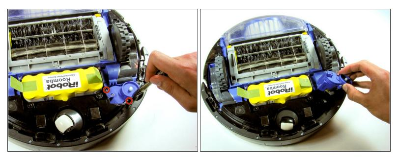
Locate and loosen the two small screws fastened to the motor housing with the Phillip's 00 Screwdriver. Like the bottom panel screws, these will not come out completely.
