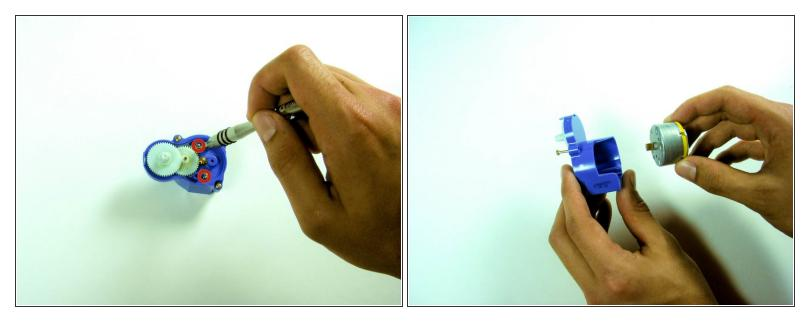
Locate and loosen the two screws inside the gearbox with the Phillips 00 Screwdriver. The motor should come right out the bottom.
