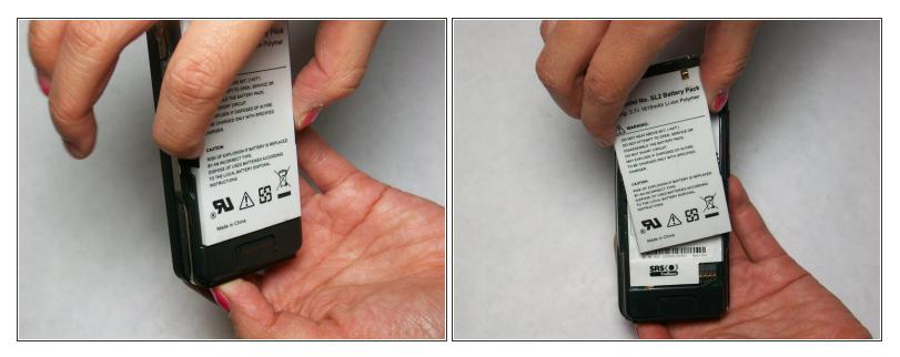
• Pinch the battery from both sides and lift the battery to remove it.
