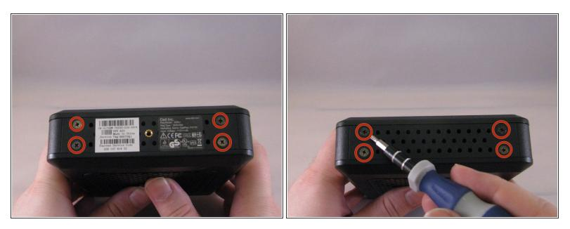
Unscrew and remove the eight 4mm Phillips #0 screws (four on top, four on bottom) from the top and bottom of the device.
