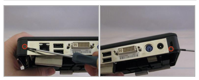
• Remove the two 4mm Phillips #00 screws that are along the back of the case.
