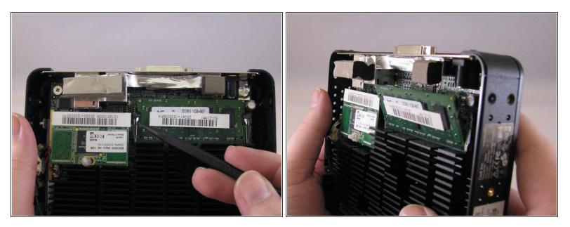
Using fingers, push the clips on either side of the RAM. The RAM will pop up at a 45 degree angle when both clips are disengaged.
