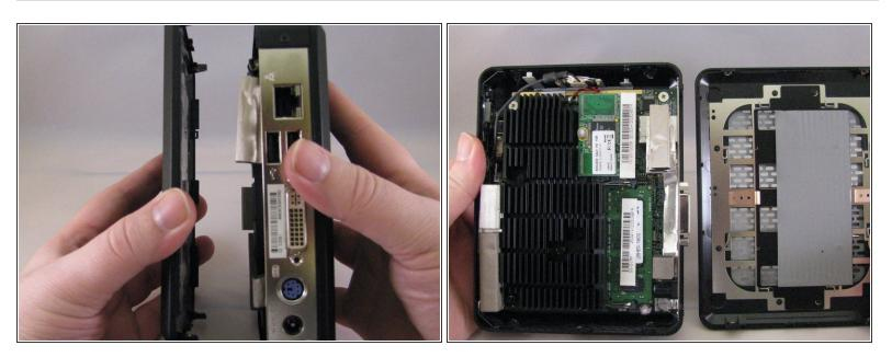
Once the clips have been released, gently disengage the cover from the rest of case by pulling in opposite directions.
