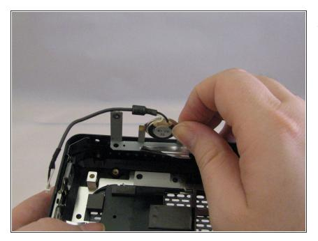
• Grasp the speaker mounting bracket and lift it up from the case.
