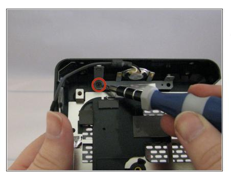
Remove the 5mm Philips #0 screw securing the speaker mounting bracket to the case.
