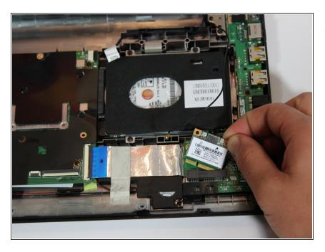
• Slide the component up and out.
