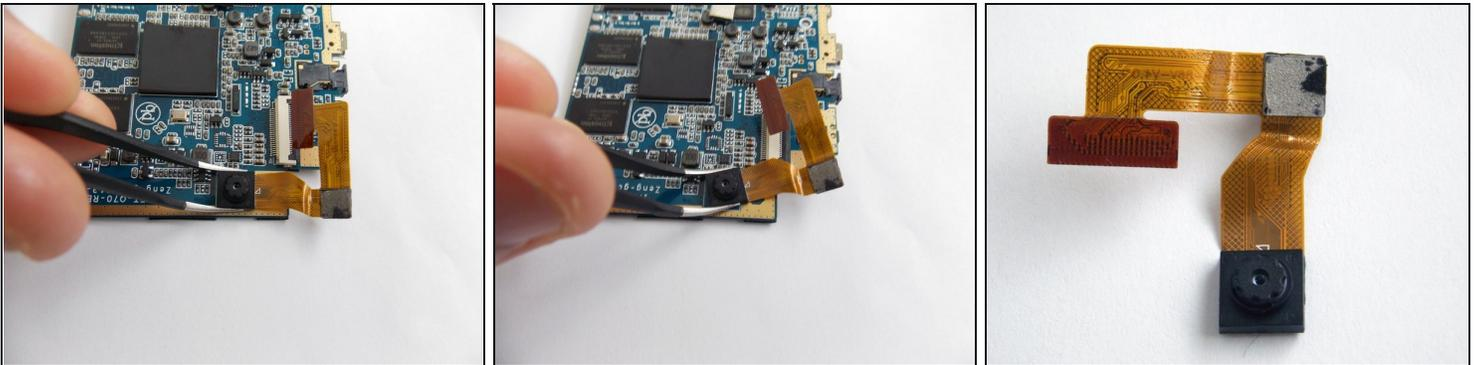
ⓘ With the power cable disconnected, the backside camera is free. However, both cameras are sequentially connected through the power cable; the front side camera is glued to the motherboard.
