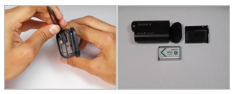
Using a pair of tweezers, firmly grip the protrusion where the PULL signifies and remove the tray and battery.
