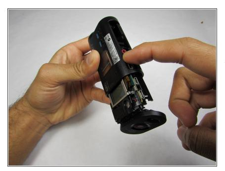
Separate the outer casing from the electronics by pushing on one of the ports toward the back end of the case. The electronics should slide right out.
