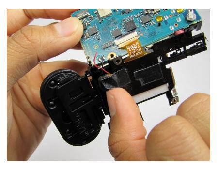
Remove the pieces of black tape holding in the speaker. Put them aside for re-assembly.
