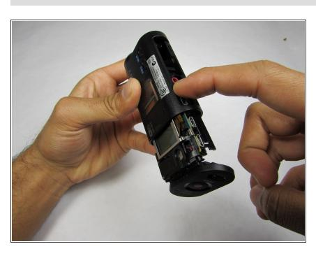
Separate the outer casing from the electronics by pushing on one of the ports toward the back end of the case. The electronics should slide right out.
