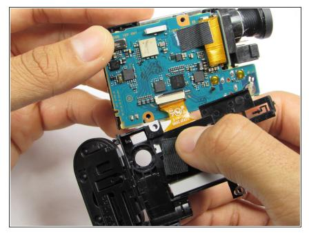
A ribbon cable attaches the LCD to the circuit board, this can be removed by gently pulling on the cable as close to the end that attaches to the circuit board as possible.
