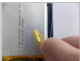
Remove the tape holding the battery in place.
