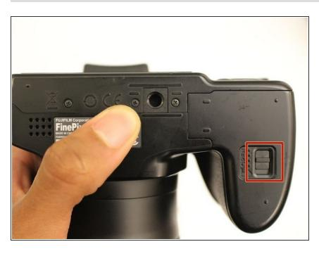
Push the battery chamber latch in the direction of the front of the camera. Keeping tension on the latch, slide the battery chamber cover toward the outside of the camera, opening the battery chamber.
