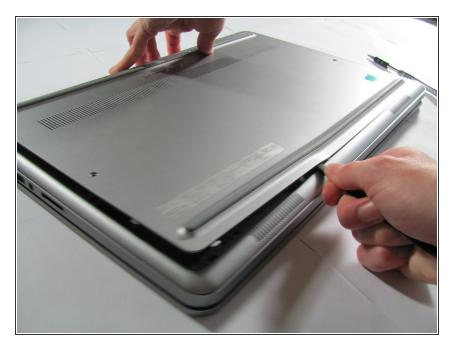
Use a spudger to remove the base cover from the rest of bottom cover.
