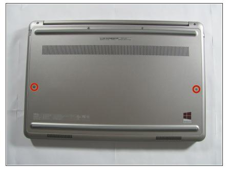
Remove the two 5 mm interior screws that connect the cover to the assembly using the same Philips head screwdriver from the previous step.
