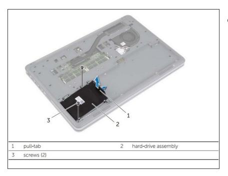
The model device did not come with a hard drive. However, you will need to remove the hard drive to proceed. Please remove the hard drive following the steps on page 16 of the official Dell Inspiron 15-7537 manual.
