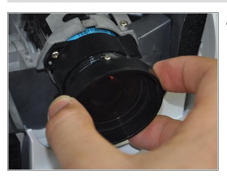
Remove the focal lens by twisting it clockwise until it comes off.
